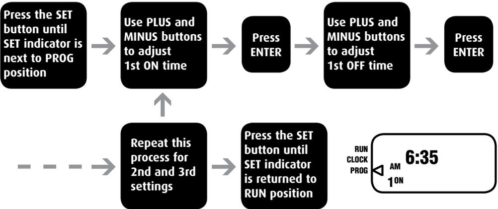
NB. The factory default settings for the 2nd ON/OFF times are both set at 12:00pm (midday) which cancels this 'ON' period giving 2 ON/OFF periods for 24hrs. If a midday 'ON' period is required set the 2nd ON and OFF times accordingly. If not press ENTER twice.
